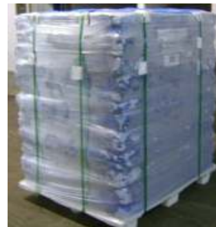
A plastic bag type “cover” is wrapped around the beef blocks, which is then secured to the pallet for loading and shipment.
